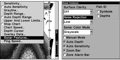
Sonar Menu with Sonar Features selected (left). In the Sonar Features menu (right), Noise Rejection is selected with ASP in the default low setting.
